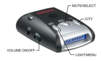
Alarms: A separate alert tone will sound for each band of Radar encountered with frequency band displayed X, K, Ka, or LASER. The signal strength indicators are 5 arrows, the stronger the signal the more arrows will display. Tone frequency will increase as signal strength becomes stronger.
